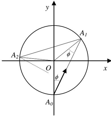
**Fig. 1** A “circular billiard”. A disc is launched from point  $A_0$  toward point  $A_1$ , where it suffers a mechanical reflection. A second perfectly elastic collision with the border occurs in  $A_2$ . The rest of the trajectory of the disc follows a similar pattern at each mechanical reflection.
