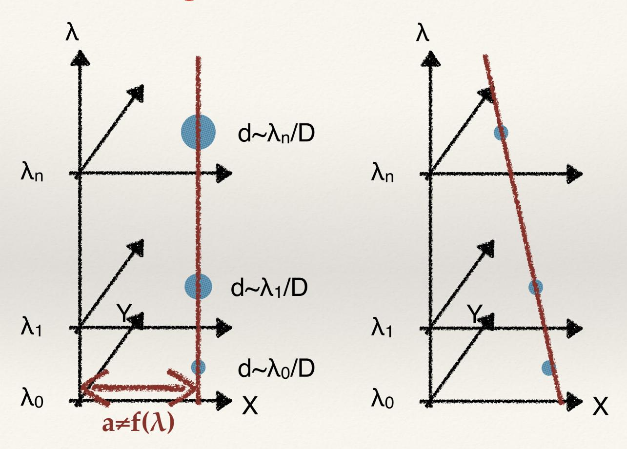
Speckle deconvolution is applicable when the planet image does not extend over the whole observed spectrum
