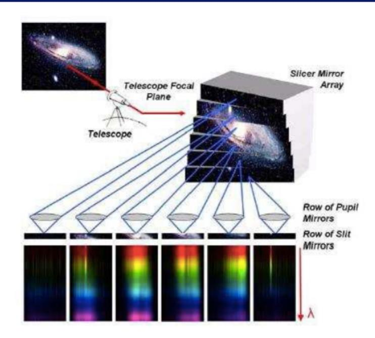
Image Slicer Spectrograph More Complex Instrument Best use of detector
